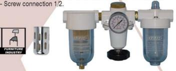
Filter + regulator + lubricant for pneumatic installations. Regulates the air pressure and oil flow required for the pneumatic tool in use, and removes the impurities in the compressed air. Technical:
