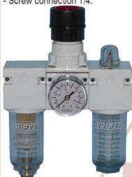
Filter + regulator + lubricant for pneumatic installations. Regulates the air pressure and oil flow required for the pneumatic tool in use, and removes the impurities in the compressed air.
