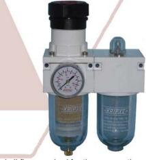
Filter + regulator + lubricant for pneumatic installations. Regulates the air pressure and oil flow required for the pneumatic tool in use, and removes the impurities in the compressed air. Technical:
